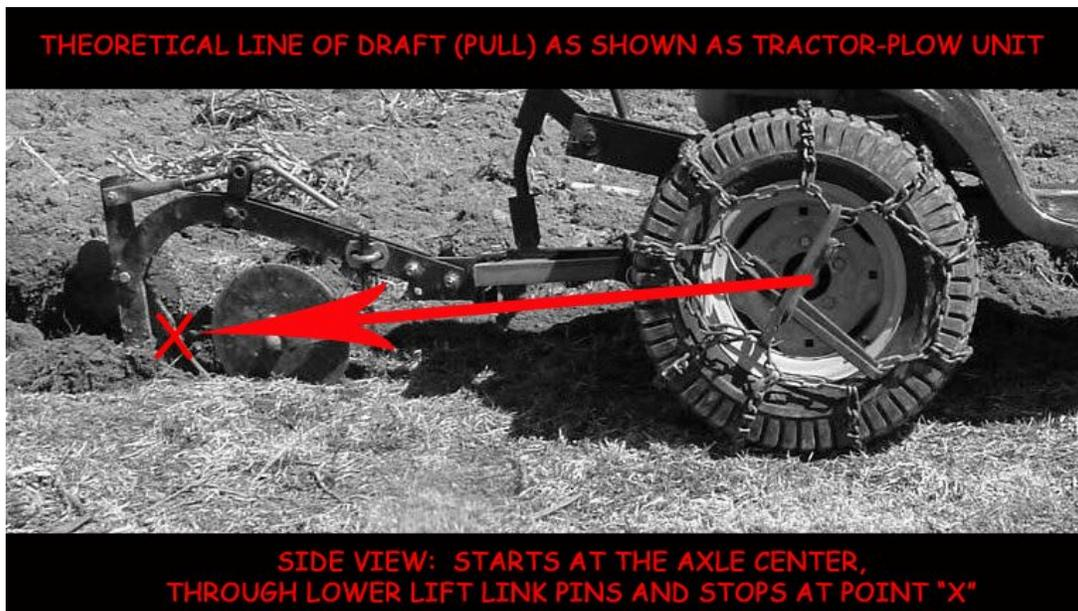
Now this all sounds technical and truly it is, but equally important. Because the imaginary center of draft must align with the center of the tractor powertrain. If not, the tractor will pull one side left or right depending on the misalignment of the plow draft center to the tractor center. Much like the struggling horse and farmer with a misaligned hitching set up, the tractor experiences the same difficulties in overcoming the tendencies of "side draft".
